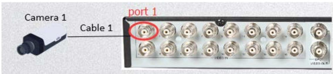
Camera 1 & Camera 2 are connected to Port 1 and Port 2 of the XVR. Camera 1 has live view while Camera 2 doesn't, problem should be within Camera 2, Cable 2 or Port 2. We can then use the Camera 1 for cross-testing.
