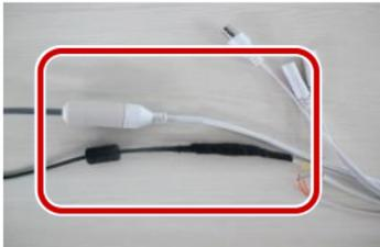
3. Protect other cables using insulating tapes.
